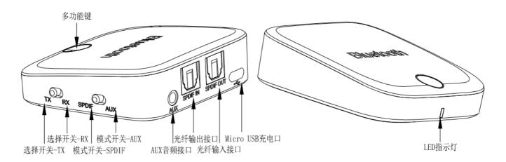
MFB (Multi Function Button), Selection Switch TX/RX (TX: transmitter; RX: receiver), Mode Selection Switch SPDIF/AUX,
